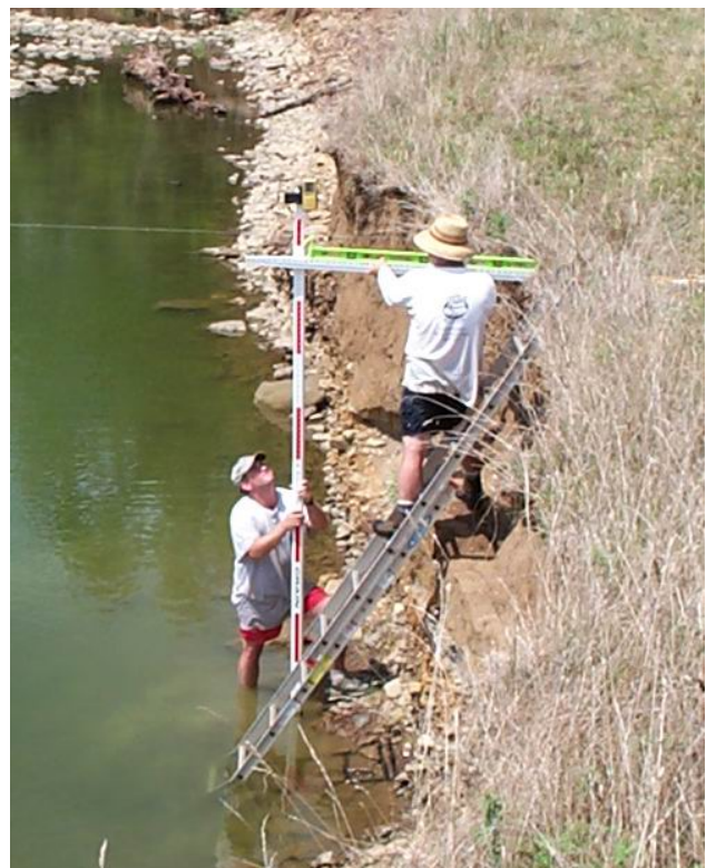
Figure 2. Measurement of lateral streambank erosion in the WFWR watershed.
